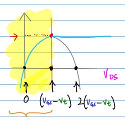
$$f(V_{DS}) = \frac{\theta}{2} \left( 2 \left( V_{GS} - V_{t} \right) - V_{DS} \right) V_{DS}$$
