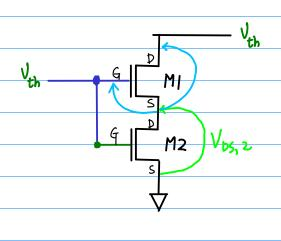
$$I_p = \frac{\beta_n}{2} \left( V_{GS,1} - V_{TOn} \right)^2$$
