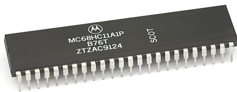
Motorola MC68HC11 in a 48-pin dual in-line package (DIP)
