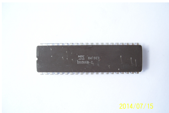
NEC \mu PD8086D-2 (8MHz) from 1984year 19week JAPAN (clone of Intel D8086-2)
