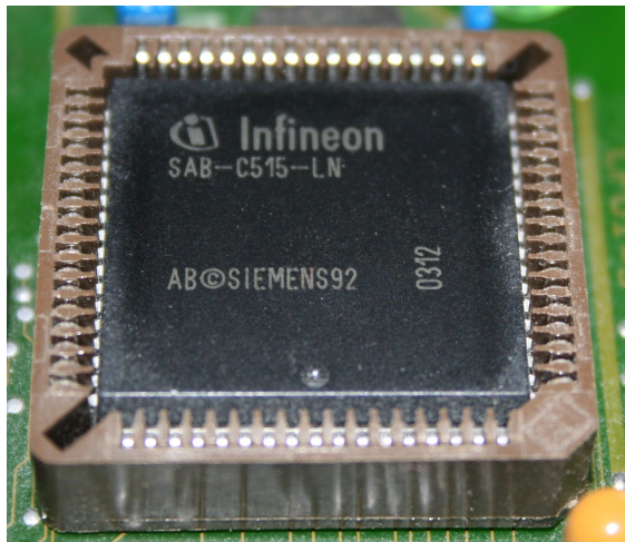
SAB-C515-LN by Infineon is based on the 8051
