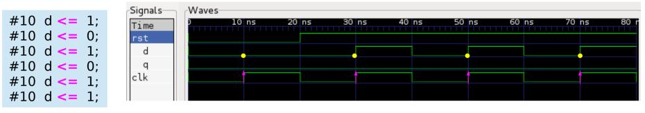
samples the <u>unchanged</u> d input values at the posedge of clk
