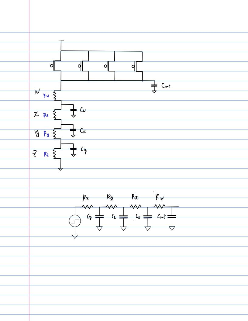
RC-Tree Pelay Model the propagation delay at node i SUM of all the time constants formed by each capacitor C, and its associated resistance Ri, k  $t_{pli} = \sum_{k=1}^{n} C_k R_{i,k}$  $R_{i,k} = \sum R_{j}$  $\Rightarrow R_{j} \in [ path(i \rightarrow s) \cap path(k \rightarrow s) ]$ common path segment from node is to source node s from node & to source node s node i : node of interest node k : 1 < k < n nodes to which capacitors are connected
