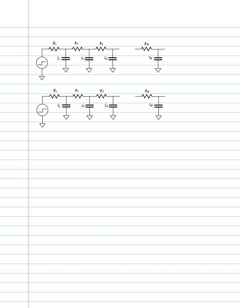
R2 Rı Rз RN ديا 🗖 **G** <u>د</u> C3 🚍  $R_1 = R_2 = R_3 = \cdots = R_N = R$  $C_1 = C_2 = C_3 = \cdots = C_N = C$ tpa= nR.c + (n+)R. C+ ... + RC  $= \frac{1}{2}n(n+1) \text{ RC} \quad \propto n^2 \text{ RC}$ • \* STC (Single Time Constant) Circuit
