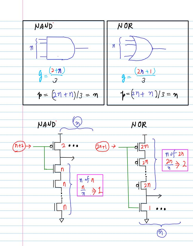
$D = N \sqrt[n]{F} + N$  $D = \sum_{i} d_{i} = D_{F} + P$ Path Delay  $= \sum_{i} f_i + \sum_{i} p_i$  $\forall i \quad \hat{f} = f_i = g_i h_i = F^{Y_N}$  equal delay  $f_1 + f_2 + \dots + f_N = g_1 h_1 + g_2 h_2 + \dots + g_N h_N$ ≥ (g, h,) (g.h) ··· (g. h) F = G HPath Effort F = GBH G = TT gi G = TT gi  $H = \frac{C_{out}}{C_{in}}$  $H = \frac{C_{out}}{C_{in}}$ 13 = 1 B = TI bi  $D = \sum_{i} d_{i} = \sum_{i} f_{i} + \sum_{i} p_{i}$ = N F <sup>1</sup>/<sub>2</sub> + N
