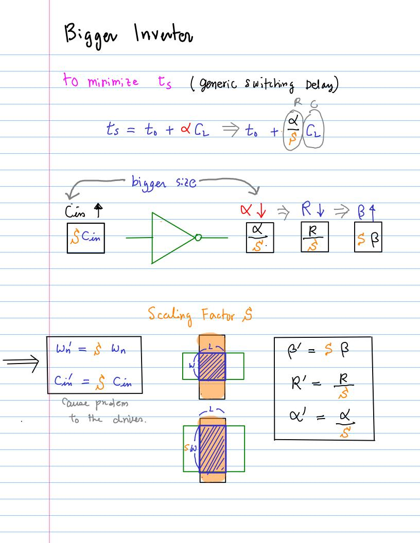
think G.P. (Geometric Progression) in Sizc factors S ⊬ Arithmetic Progression >/ Geometric Progression min delay Z path delay when all equal path delay
