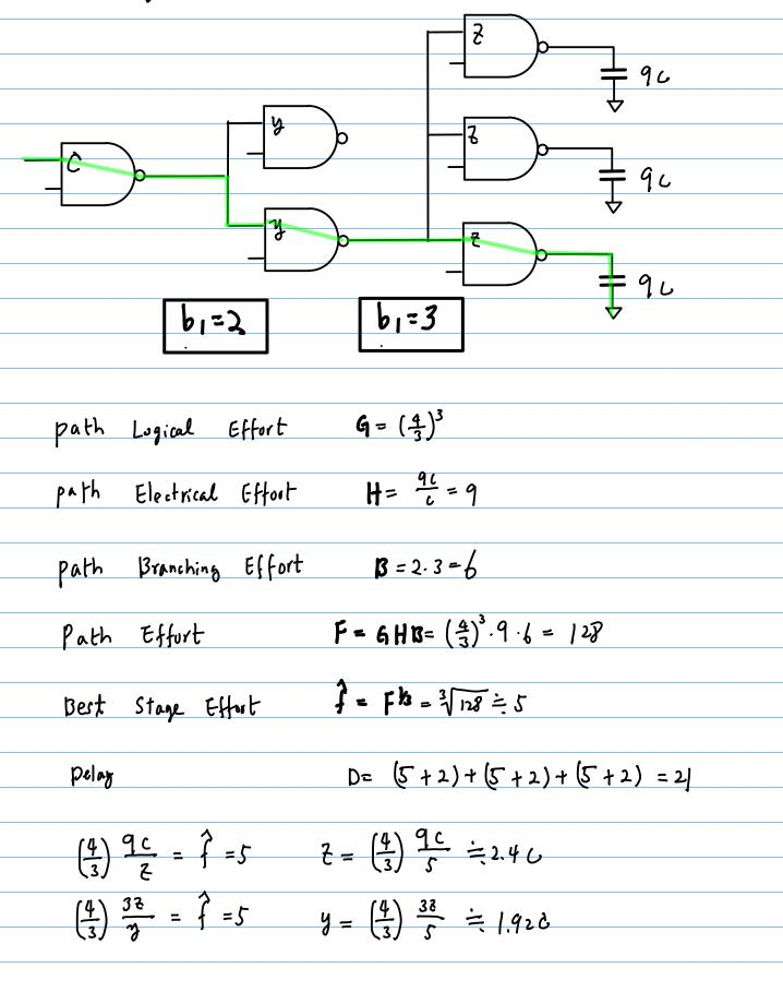
Ex2) BGH 2 :90 y 2 ± 90 Y = 96  $G = (\frac{4}{3})(\frac{4}{3})(\frac{4}{3}) = (\frac{4}{3})^3 = -0 - \frac{(2+n)}{3} = \frac{4}{3}$  $= \frac{qc}{c} = q$ H qc  $B = \begin{pmatrix} \frac{2^{1}}{3} \\ \frac{3^{2}}{3} \end{pmatrix} \begin{pmatrix} \frac{3^{2}}{2} \end{pmatrix} = 2 \cdot 3 = 6$ C  $F = BGH = 6 \cdot \left(\frac{4}{3}\right)^3 \cdot 9 = 2 \cdot 7 \cdot \frac{4^3}{2^3} \cdot 9 = 128$
