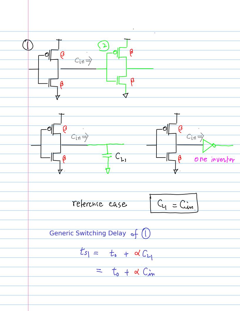
When CL >> Cin many inverters ୧ b ٠ 0 0 to minimize ts (generic switching Delay)  $\forall \downarrow \Rightarrow R \downarrow \Rightarrow \beta \uparrow \Rightarrow bigger size$ speed V.S. area tradeoff  $t_s = t_0 + \alpha C_L$   $t \approx RC$  $(\chi \propto \frac{1}{\beta(V_{pp}-V_{T})})$ CL
