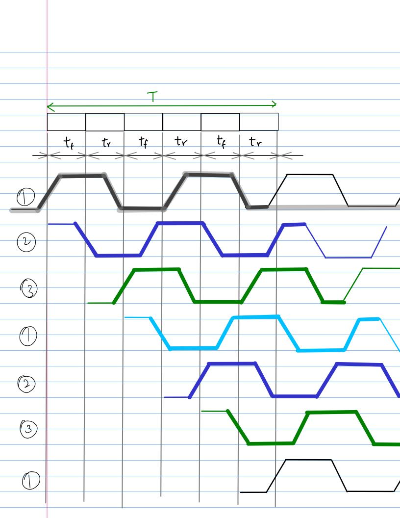
$T = 2 \cdot t_{P} \cdot N$ tp: propagation dulay N: # of inverters in chain T>> tf + tr - used to measure the average propagation delay of a typical inverter with minimum Capacitive Loading  $t\rho = \frac{1}{2.N}$ Characterise a particular design/fabrication process - used as a simple on chip clock
