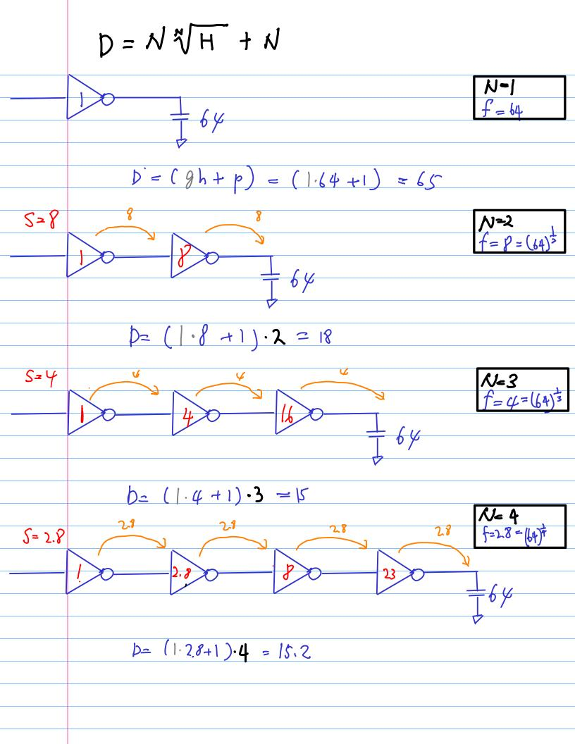
N Stages  $\leftarrow$ n₁ stages N-n₁ stages  $D = g_1h_1 + g_2h_2 + \dots + g_Nh_N \ge (g_1h_1)(g_2h_2) \dots (g_Nh_N) = GH = F$  $g_1h_1 = g_2h_2 = \cdots = g_Nh_N = F^{N_N} \rightarrow minimum$  $D = N F^{N} + \sum_{i=1}^{n_i} p_i + (N - n_i) P_{iN}$  $p_i$ : i-th stage parasitic capacitance  $(1 \le i \le n_i)$ pinvi inverter "" ( $n_i+1 \le i \le N$ )
