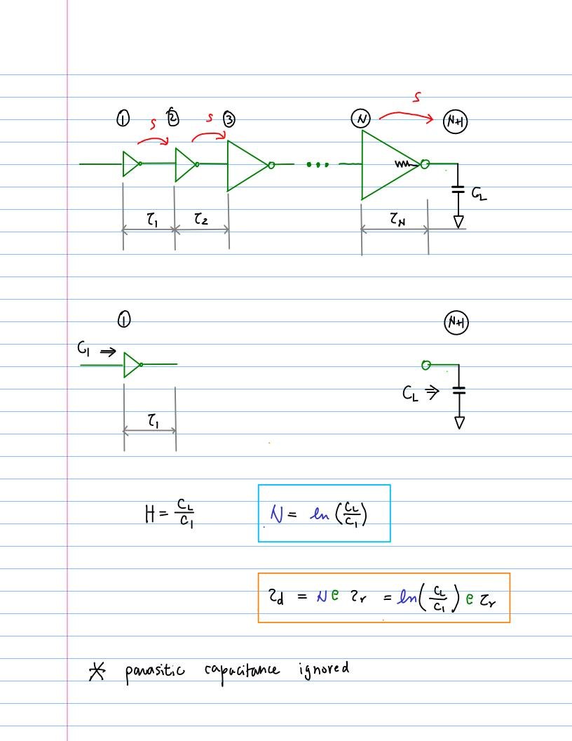
Ignoring Cpm  $C_1 \Rightarrow$  $C_2 \Rightarrow \frac{1}{6} 6 \%$  $N = ln\left(\frac{c_{\rm L}}{c_{\rm 1}}\right) = ln\left(64\right) = 4.15 \Rightarrow N=4$  $Z_d = ln\left(\frac{c_L}{c_1}\right)SZ_r = Sln(64)Z_r (Z_r)=R_1C_1$  $S = \left(\frac{CL}{C_1}\right)^{\frac{1}{N}} = 64^{\frac{1}{4}} = \frac{2.8}{2}$  $= 64^{\frac{1}{4.15}} \Rightarrow C = 2.018$ 28 رگ  $\mathcal{J}$ ンる 28=784  $2.8^3 = 21.95$ Zd= 2.8 In (64) Zr = 11.6 Zr
