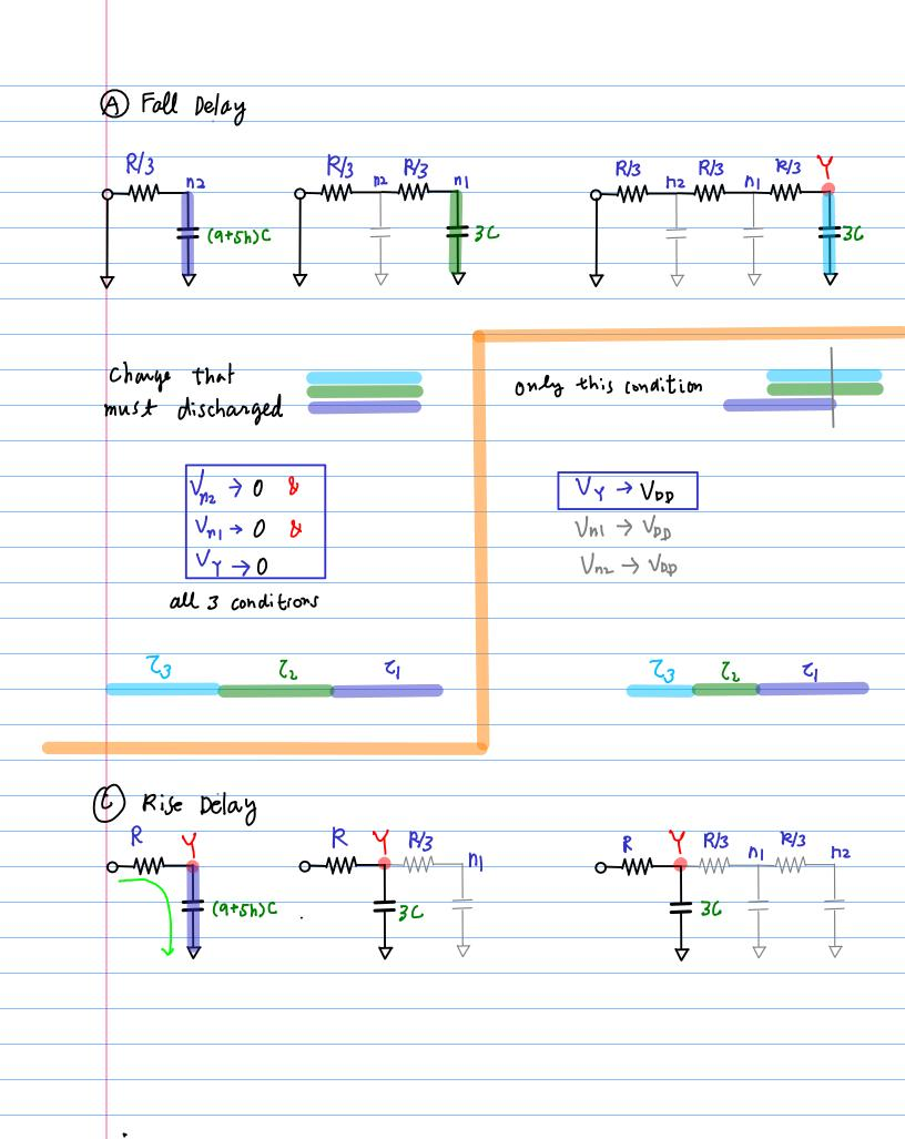
Input Transitions for a Minimum Delay Rise ₿ ABC = (A+B+C)=13 current sources Simultaneous falling to charge CL \_ Fall ABC=1One input rising lately Only have to discharge other inputs the parasitic capacitance already "H" of one nmos transistor Smallest resistance. this lately rising input is feed to the n Mos that is close to Y
