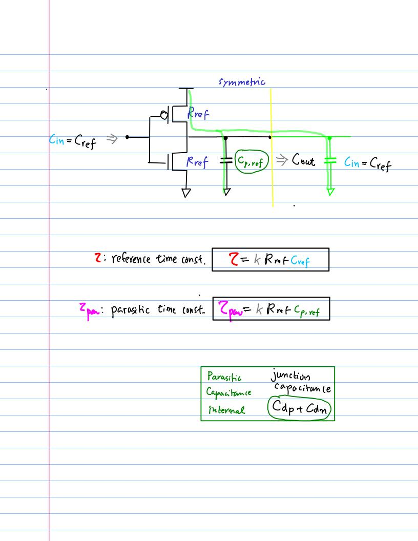
Electrical Effort  $h = \frac{C_{out}}{C_{in}}$ Panasitic Delay  $p = \frac{2pan}{2} = \left(\frac{kRref}{kRref}\frac{C_{p,ref}}{C_{ref}}\right) = \left(\frac{C_{p,ref}}{C_{ref}}\right)$ Symmetric Rref d Cin=Cref > •  $Rref = C_{p,ref} \Rightarrow Cout = = C_{ref}$ Zpur 7
