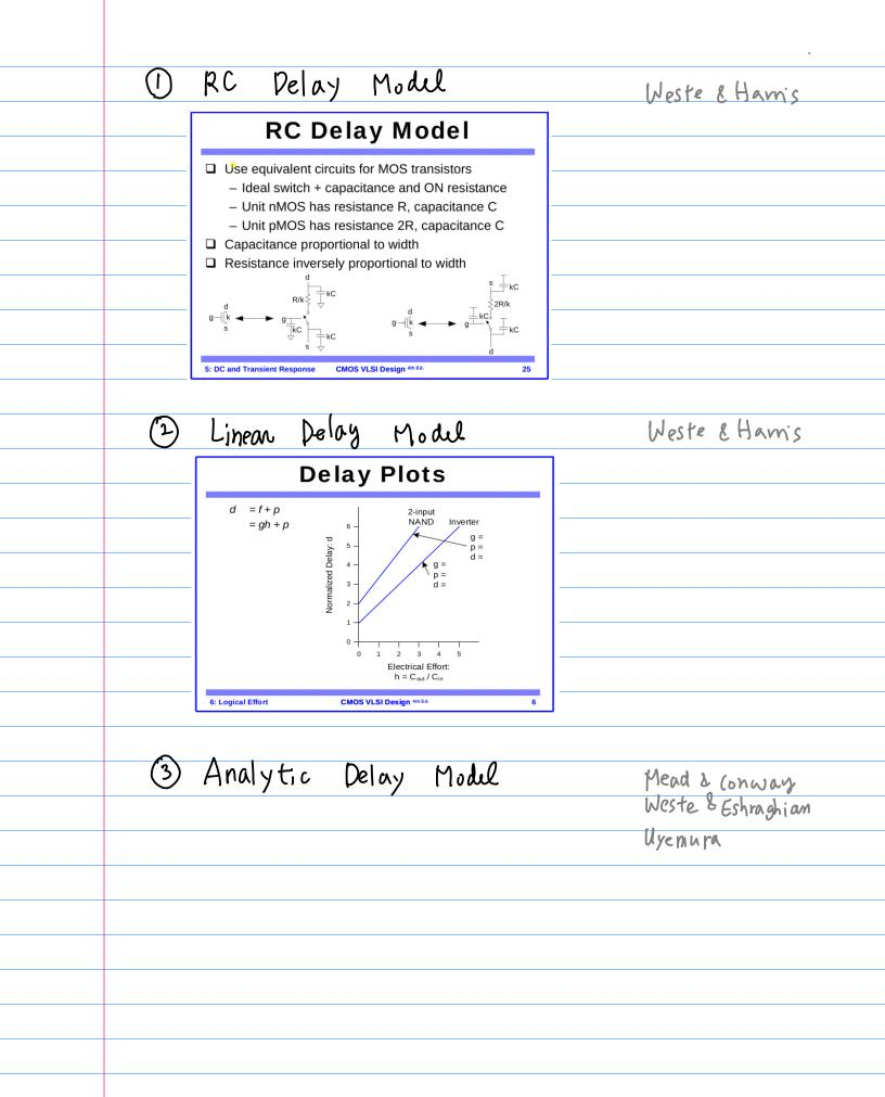
**Inverter Delay** for every kind of inverter g = 1 Cout Normalized Delay  $d = (p + g \cdot (k)) = (p + (k))$ = dabs Absolute Delay dabs = Zref (p+h)
