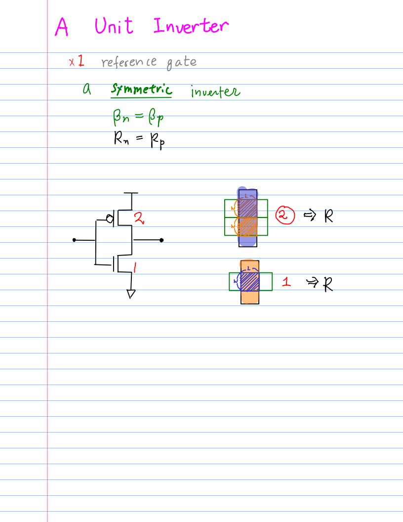
Sizing, Scaling d <u>4</u>7 4 x ref IX ref the smallest sizing in the logic chain  $\left(\frac{\omega}{L}\right)_{p} = r \left(\frac{\omega}{L}\right)_{m}$  $\left(4\frac{W}{L}\right)_{p} = r \cdot \left(4 \cdot \frac{W}{L}\right)_{m}$ for the same L,  $\left(\frac{4W}{L}\right) = \mathcal{V} \cdot \left(\frac{4W}{L}\right)_{m}$ 4 4 Large Drive Strength
