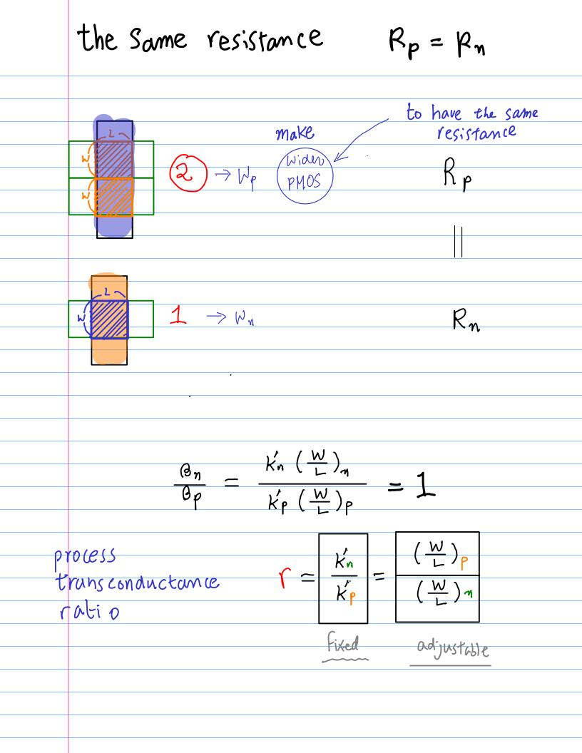
as pect ratio for the same (R) a symmetric inverter Bn = Bp Rn = Rpa relative aspectiratio d  $(\beta_p) = (\beta_n) \quad r = 2 \sim 3$  $\left(\frac{\omega}{L}\right)_{p} = r \left(\frac{\omega}{L}\right)_{m}$  $Kn = r K_p$ for a fixed (h),  $W_{p} = \bigvee_{n} W_{n}$ consider a scale factor
