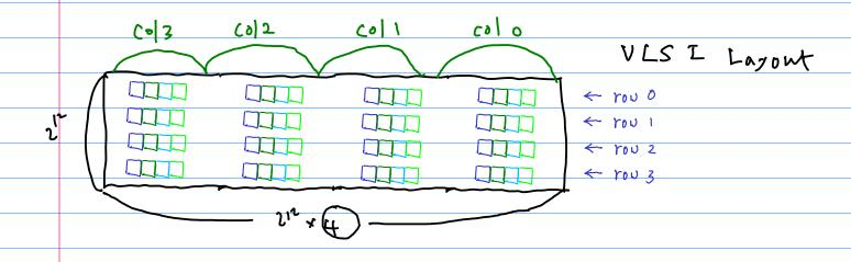
64Mbit (16Mx4bit) DRAMe17主 4096 columns 46:6 4 bib/column RAS Sense amp data bus 12-bit YOU YOW 4091 addy add Mux de cod into buf -4096X4-DRAM refresh Col addr deader CAS col. addr buf RAS Mux 12-bit [A23~A12] A11~A0 12-617 3 CAS 24-bit andress
