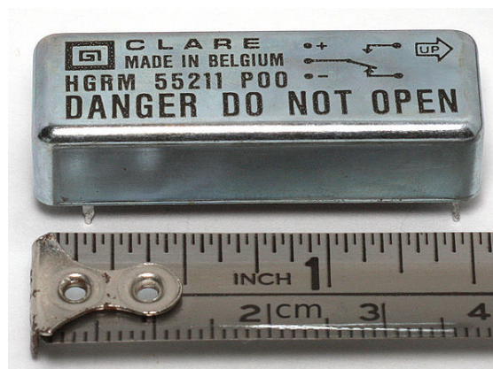
A mercury-wetted reed relay that has AC/DC switching specifications of 100 W, 500 V, 2 A maximum
