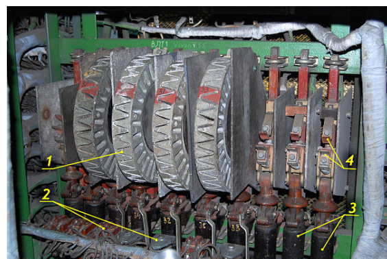
Powerful DC contactor with electro-pneumatic drive
