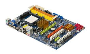
A motherboard with integrated graphics, which has HDMI, VGA and DVI outs.
