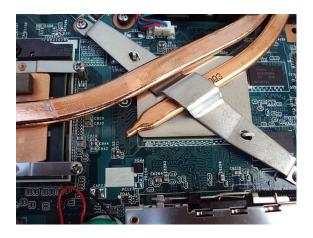
The ATI HD5470 GPU (above) features UVD 2.1 which enables it to decode AVC and VC-1 video formats
