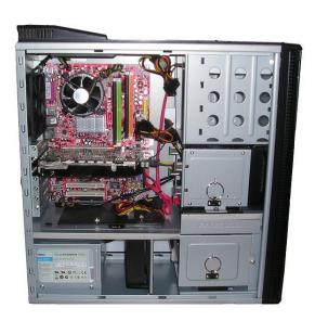
Inside a custom-built computer: power supply at the bottom has its own cooling fan.
