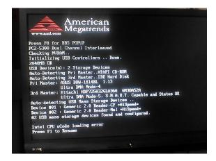
An American Megatrends BIOS showing a "Intel CPU uCode Loading Error" after a failed attempt to upload microcode patches into the CPU.
